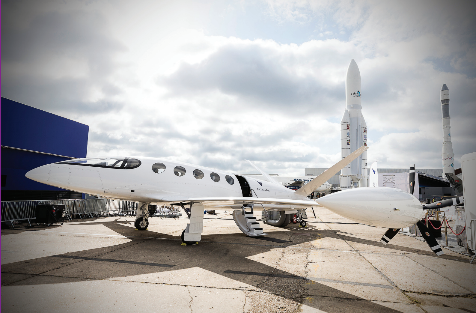
Israeli firm Eviation launched their electric aircraft – named Alice – at the Paris Airshow in 2019. They say the craft will carry nine passengers for up to 650 miles at 10,000ft at 276mph. It is expected to be launched in 2022 (Picture Source: Eviation media kit)
